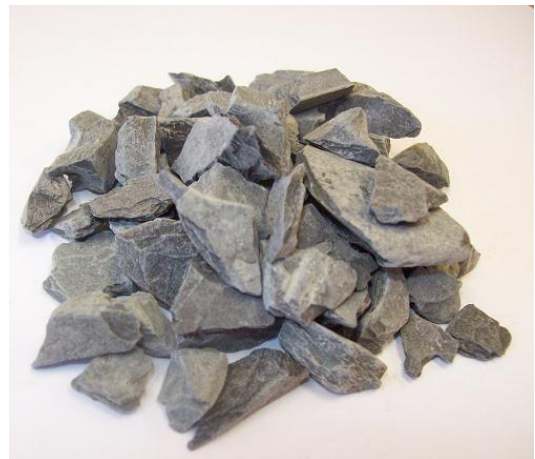
Figure 2. Drilling cuttings from deep-seated geological structure (Paleozoic) in Pomerania (Poland)
