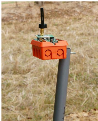
Figure 1. A Sensor node installed over station
